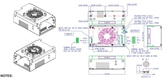
Input Connector(CN3): Mating Molex Part No. 09-91-0500 or equivalent (5 pin, 3 used) PCB Labeling: L = Line; N = Neutral; G = Chassis Ground; Molex Engineering Series 2478, 2578, 8818 or Howder M3. 3 pin Terminal block 6.35MM Center (HD-601-3P).
